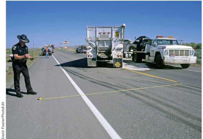
Figure 16-14 In a multiple-car collision, skid marks can help to determine the path and speed of each vehicle.
